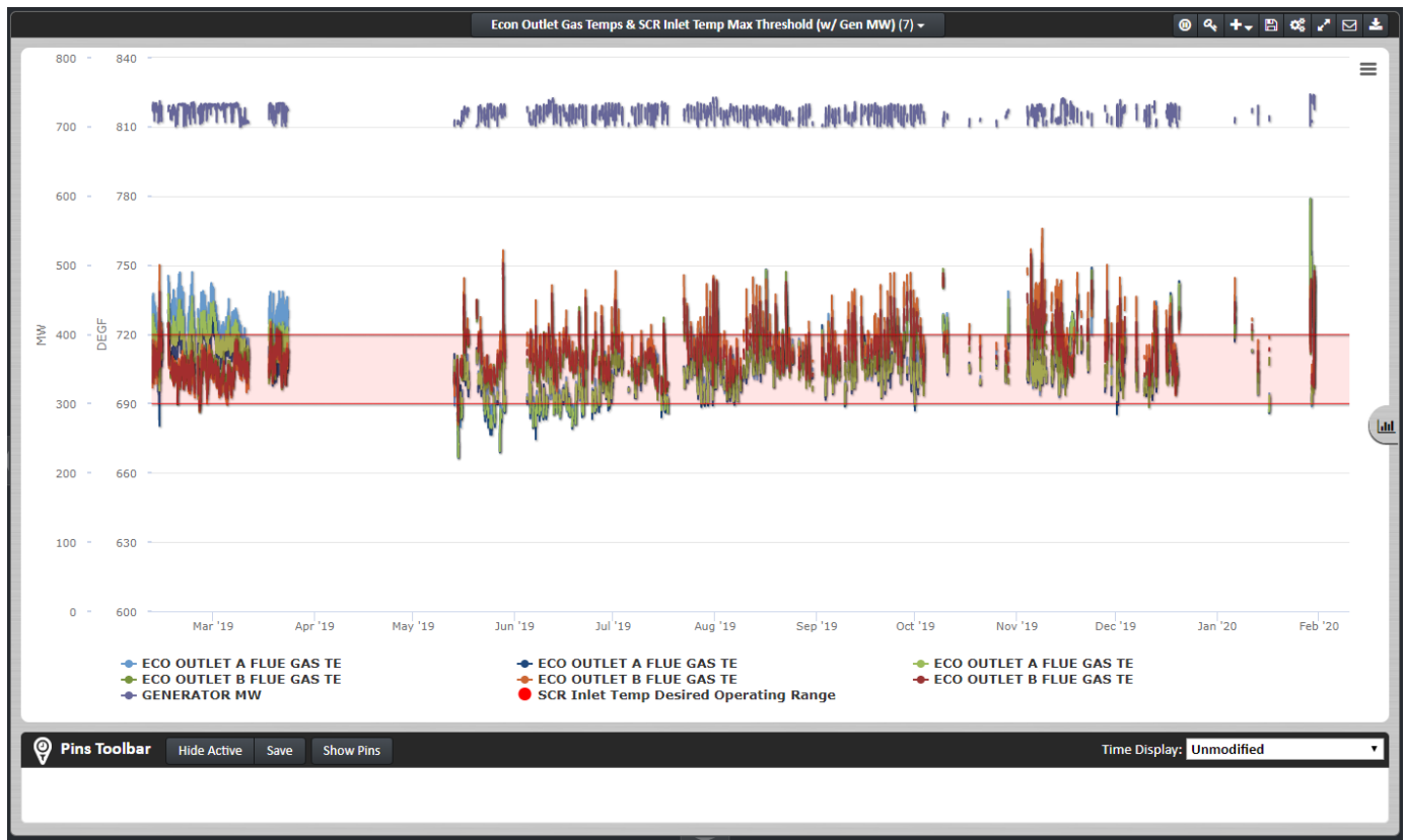
Figure 3-17 Plum Point SCR Inlet Gas Temps Filtered for High Load (Hourly Averages)
