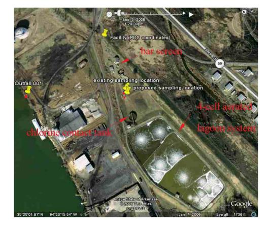
Existing 3.1 mgd treatment system before construction of new plant started:
