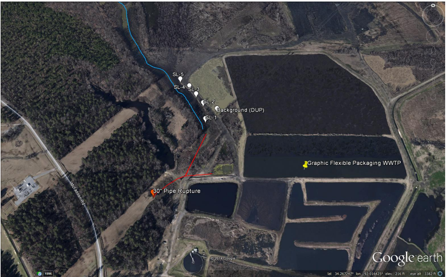
Figure 1. Google Earth image dated Feb 2, 2013 showing surrounding area and sample locations. Red line - direction of SSO. Blue line – unnamed slough.
