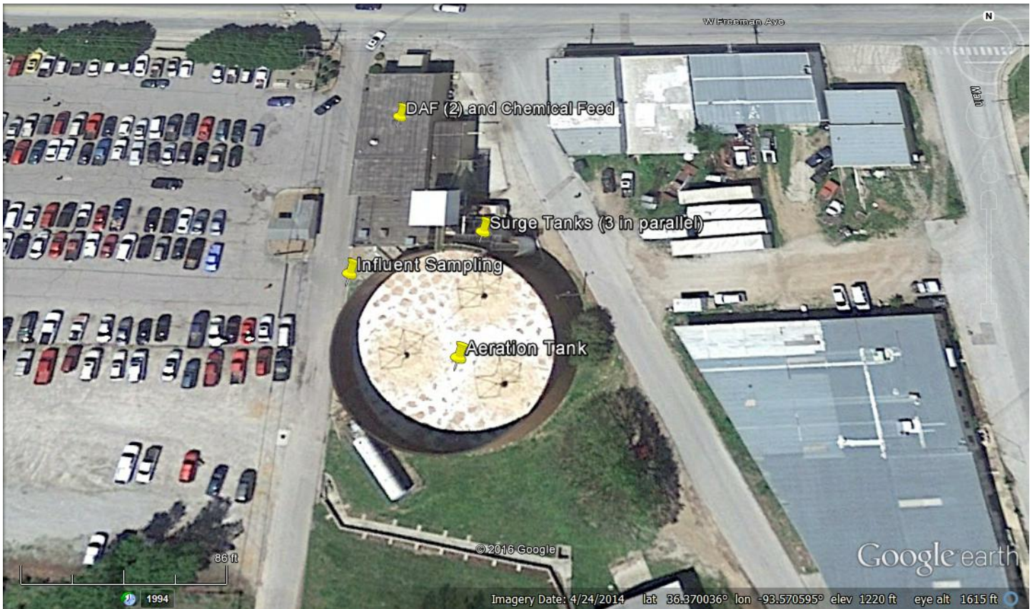
Figure 1. Google Earth image dated April 24, 2014 of the Tyson – Berryville pretreatment plant with major components identified.
