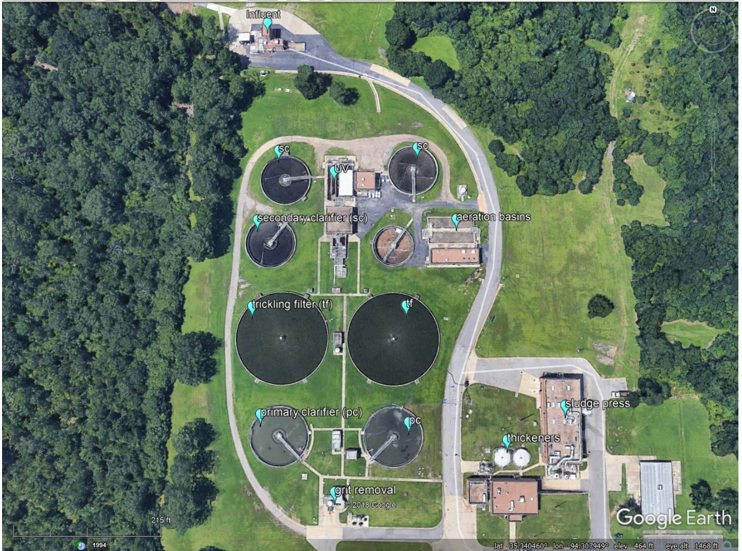
Figure 1. Google Earth image (not dated) showing facility overview and major treatment components.
