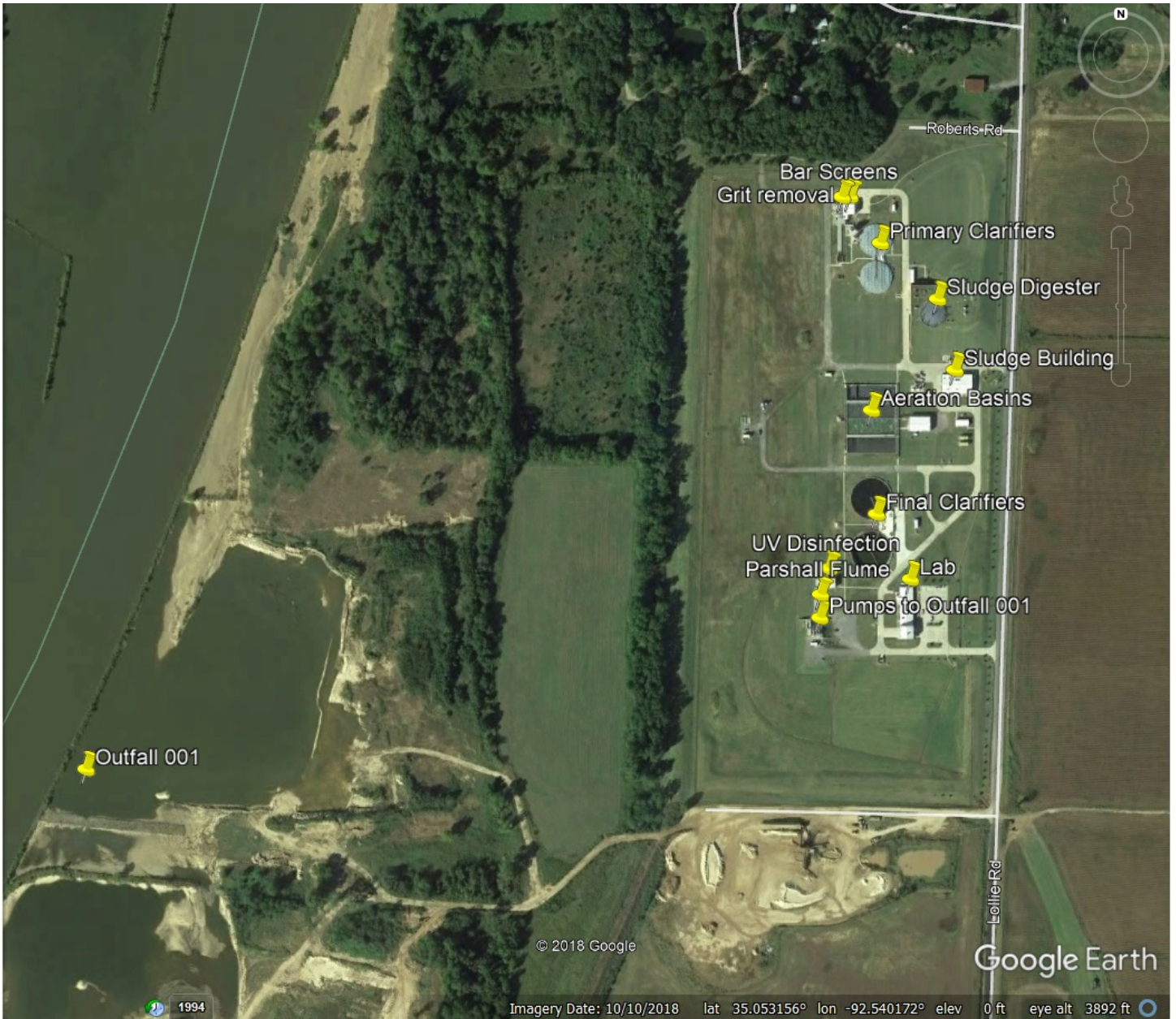
Figure 1. Google Earth image dated October 2018 showing components of the facility's treatment system.
