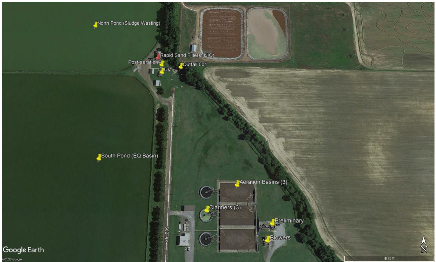
Figure 1. Google Earth image dated June 7, 2106 depicting City of Forrest City POTW with major components identified.
