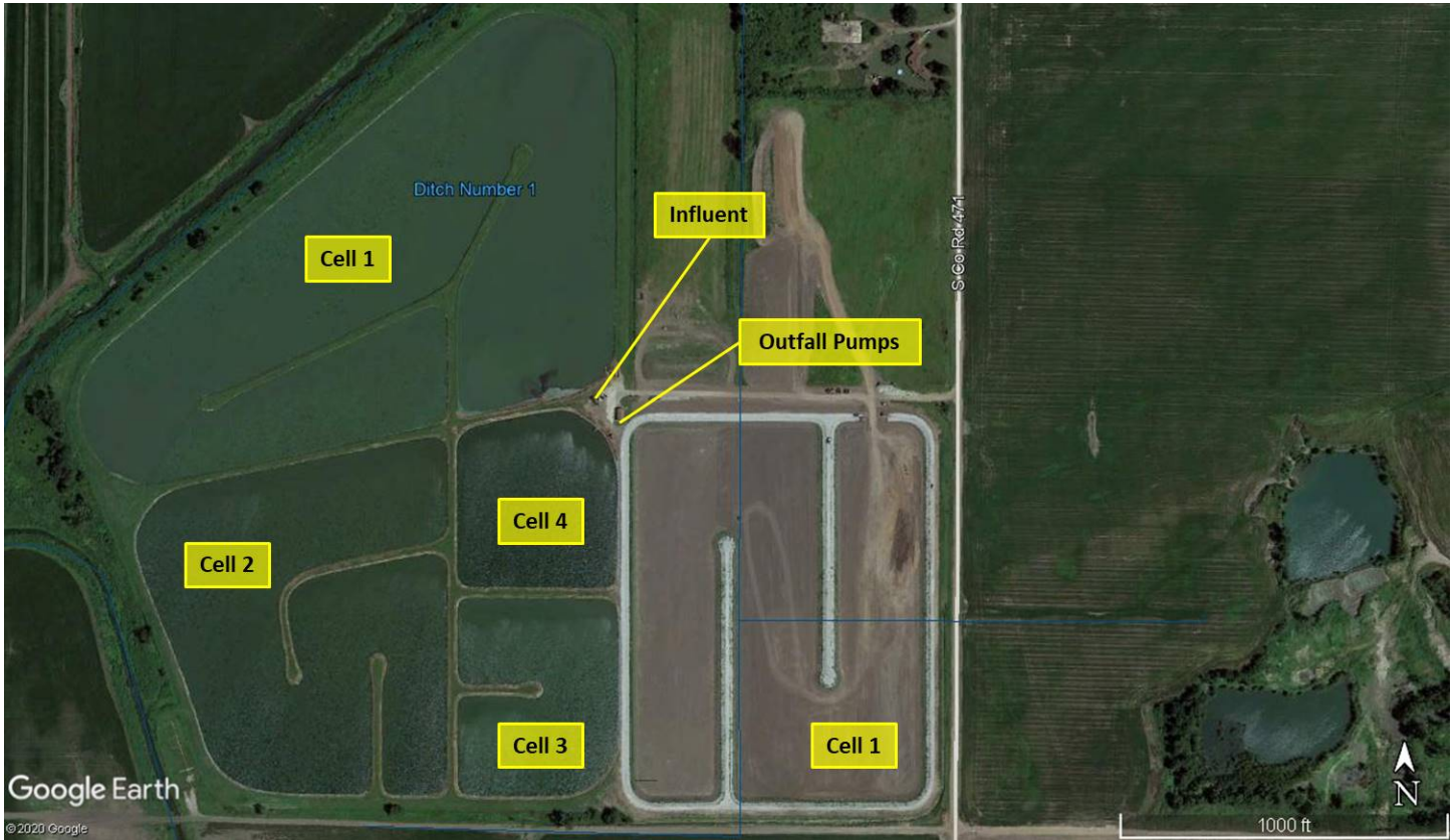
Figure 1. Google Earth image of the City of Osceola WWTP with labels for the different areas of treatment.
