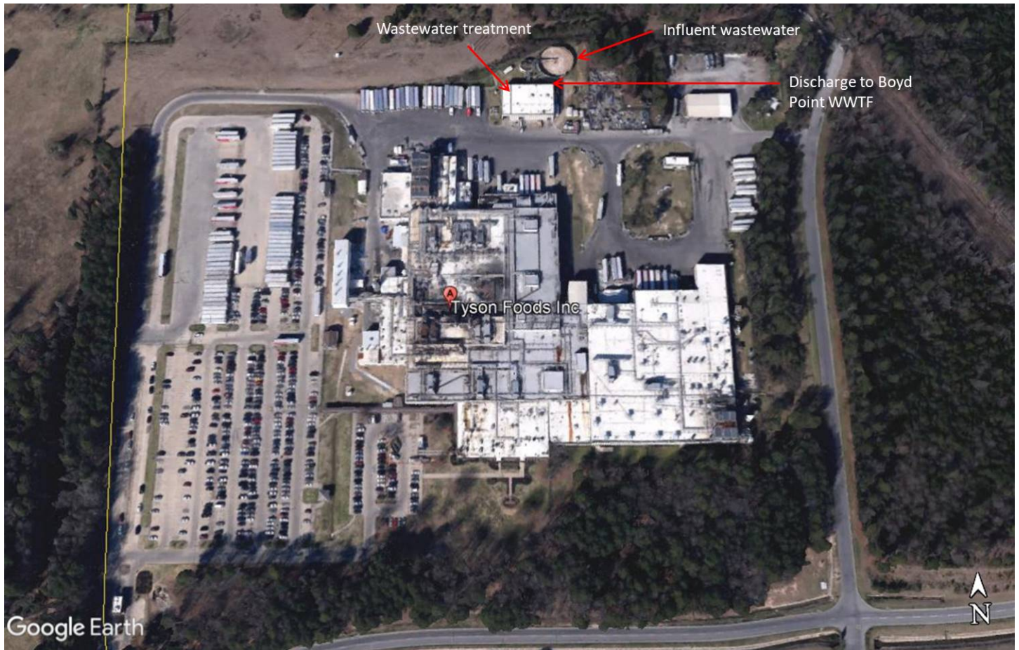
Figure 1. Overview of Tyson Foods, Inc. – Pine Bluff Poultry Plant with the locations of the wastewater treatment units indicated.
