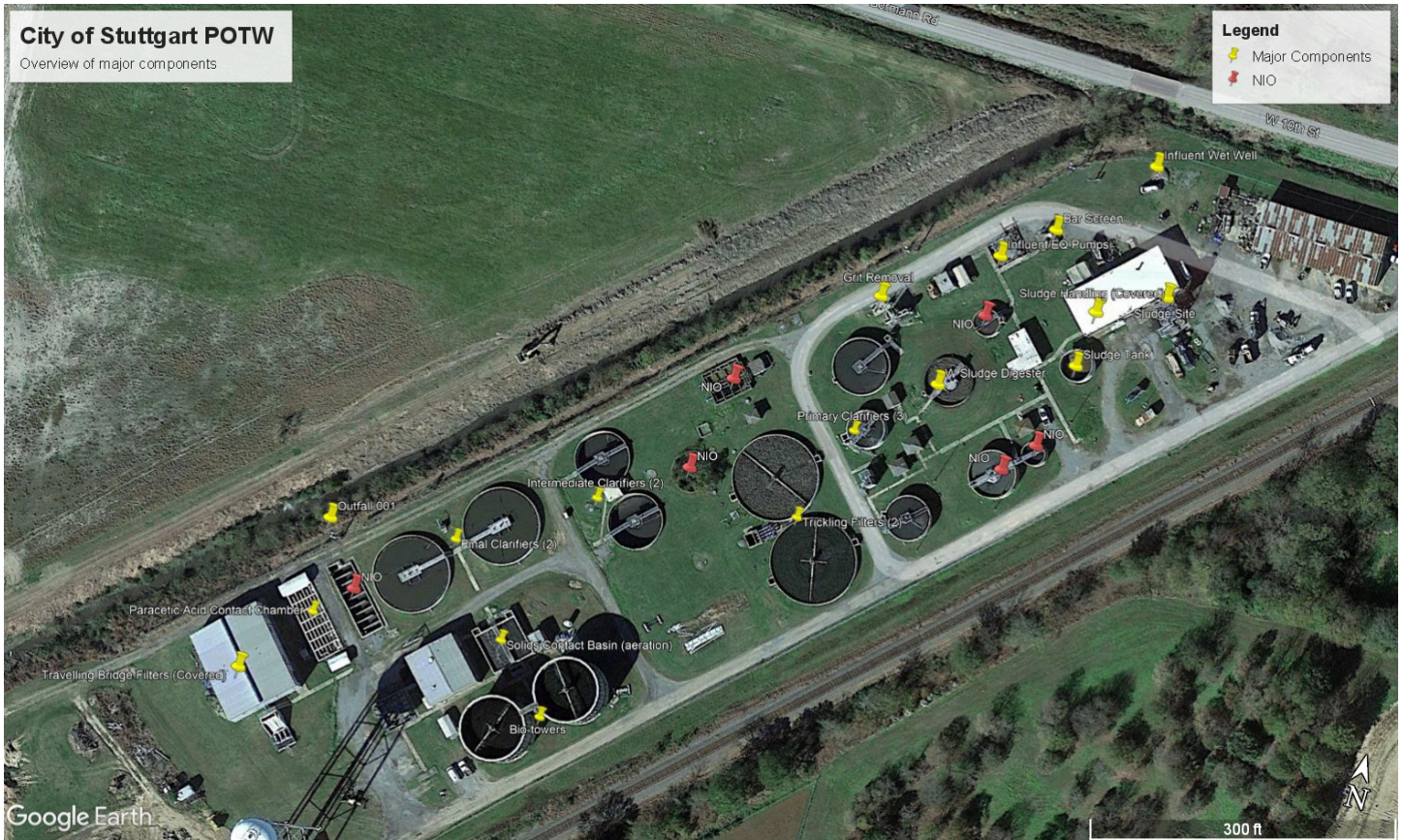
Figure 2. Google Earth image dated Nov 2020 depicting the City of Stuttgart POTW with major components identified. Red pins are components that are not in operation (NIO).
