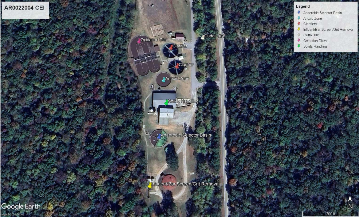
Attachment 1. Google Earth satellite imagery depicting the City of Huntsville Wastewater Treatment Facility and identifying parts of treatment.
