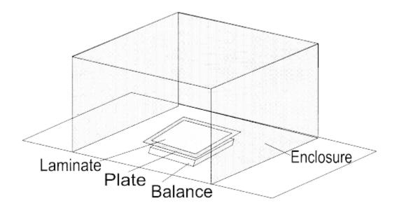
Figure 17.1. Typical Balance Enclosure
