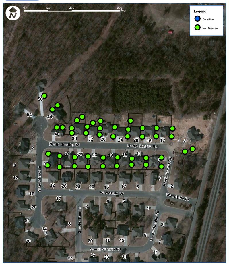
The above locations were monitored for Benzene, VOC, and H2S at the beginning of the night work shift 4/15/2013. All readings were below the limit of detection for the instruments used.
