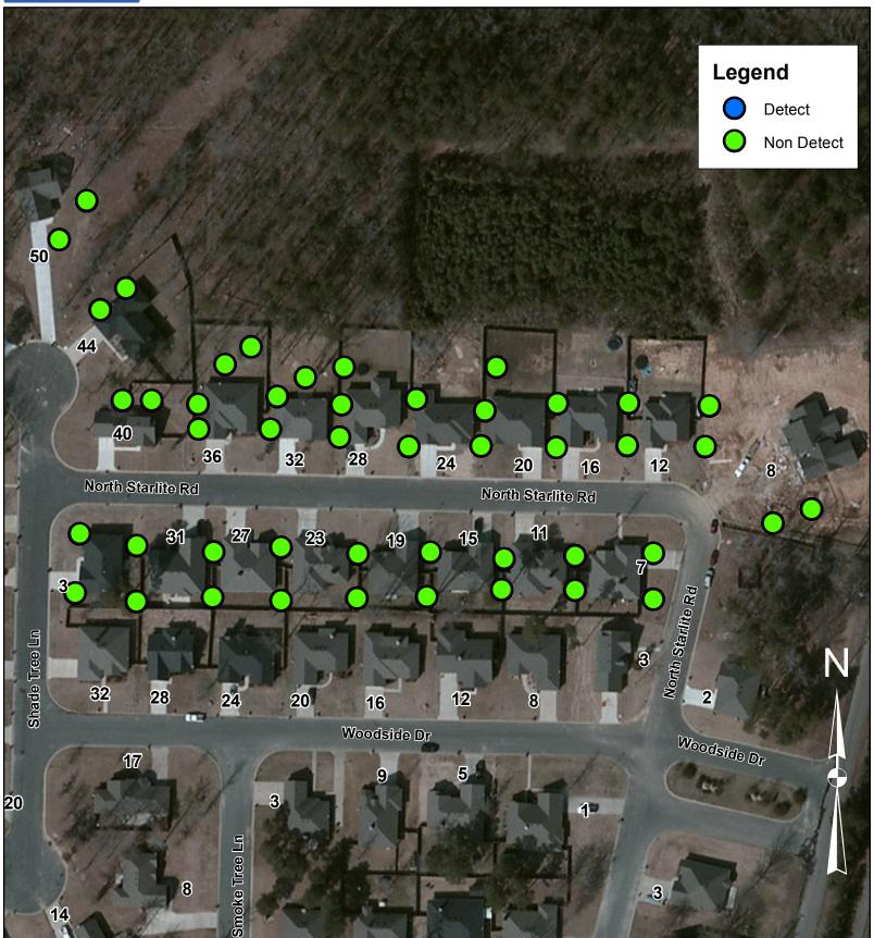
The above locations were monitored for Benzene, VOC, and H2S during the day work shift. All readings were below the limit of detection for the instruments used.
