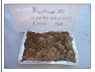
0.0 – 0.5 ft GRAVELLY SAND (SP), some fine sand, fine to medium grained sand, coarse subangular gravel, brown, moist, no odor
