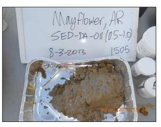
**0.5 – 1.0 ft** CLAYEY SAND (SC/CL), soft, fine grain sand, low plasticity, wet, no odor
