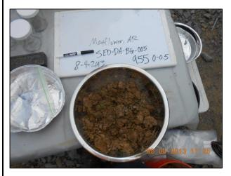
0 – 0.5 ft CLAY (CL), some silt, soft, medium to high plasticity, dry to moist, no odor
