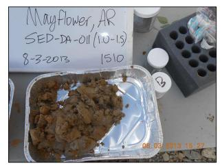
**1.0 – 1.5 ft** CLAYEY SAND (SC/CL), soft, fine grain sand, low plasticity, wet, no odor
