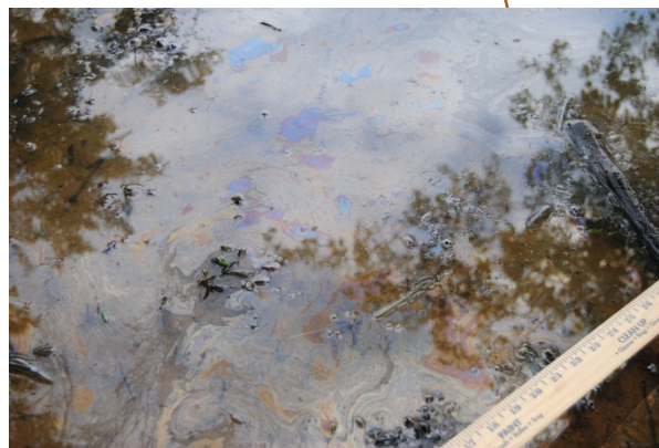
Rainbow Sheen Patch/Streamer with Oil Spot (0.1- to 0.5-inch Wide) Observation on 05/22/2014
