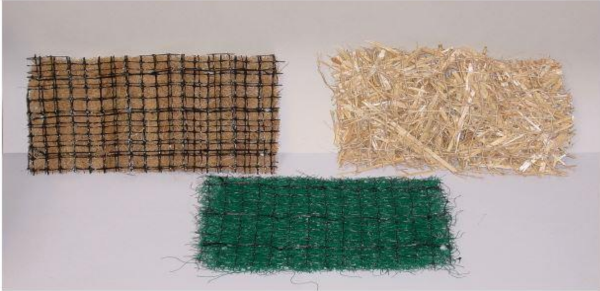
Figure 4-13: Erosion control mats
