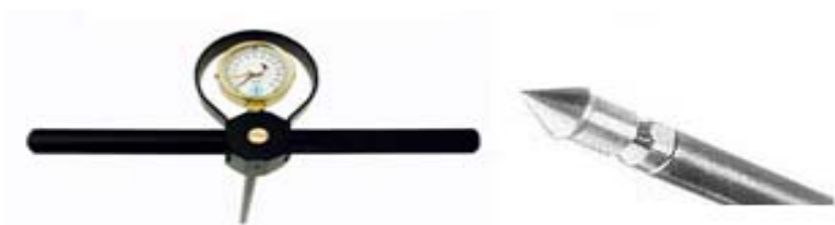
Figure 3.4. Static cone penetrometer used to measure sediment thickness in Lake Conway.
