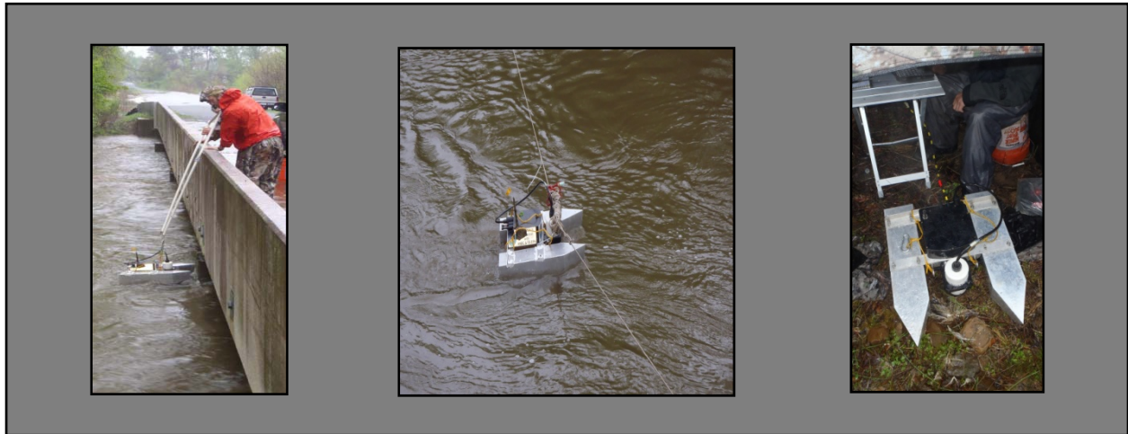
Figure 3.3. Use of ADCP during high-flow conditions.
