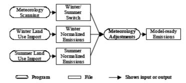
Figure 2-2. Flow diagram of SMOKE/BEIS2 processing steps.
