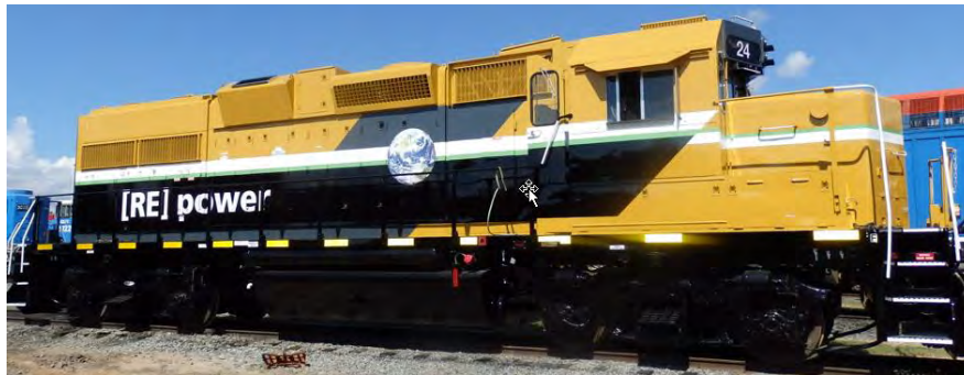
Remanufacture Switch Locomotive EMD24 to Tier 4
