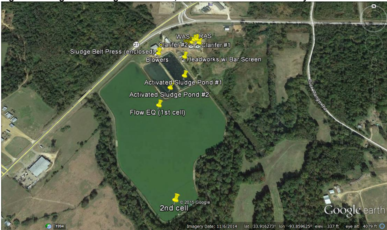
Figure 2. Google Earth image dated Nov 6, 2014 of the older components of the City of Nashville's WWTP that have been repurposed.
