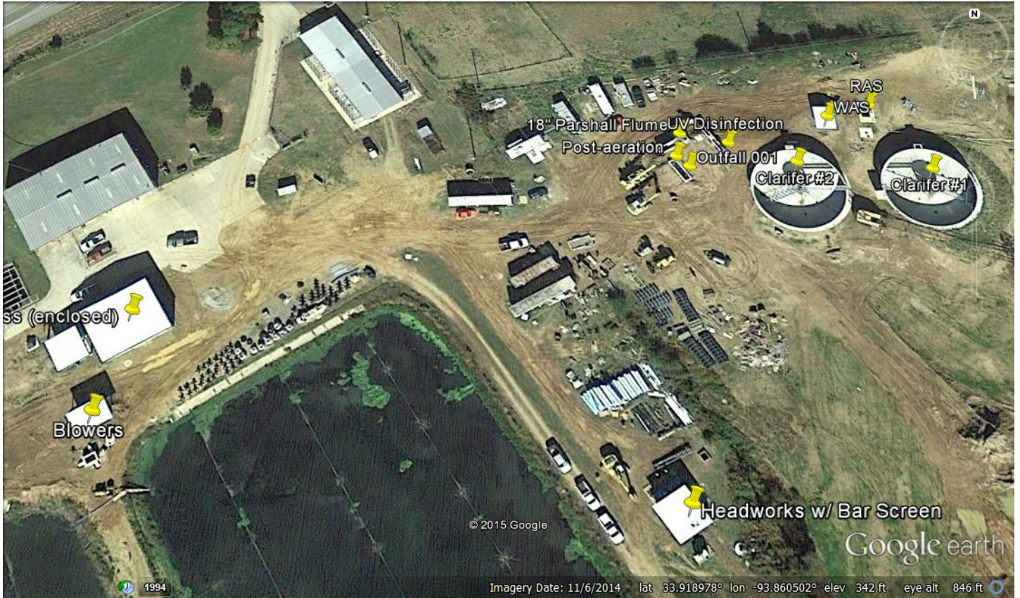
Figure 3. Google Earth image dated Nov 6, 2014 of the newer components of the City of Nashville's WWTP.
