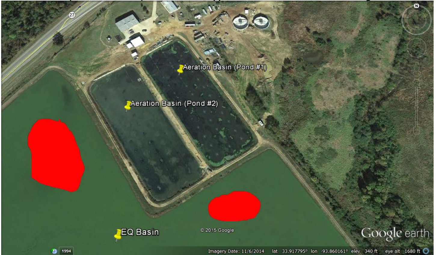
Figure 1. Google Earth image dated Nov 6, 2014 showing the converted three-cell lagoon into two aeration basins (Ponds #1 and #2) and EQ basin; approximate size and location of sludge islands.
