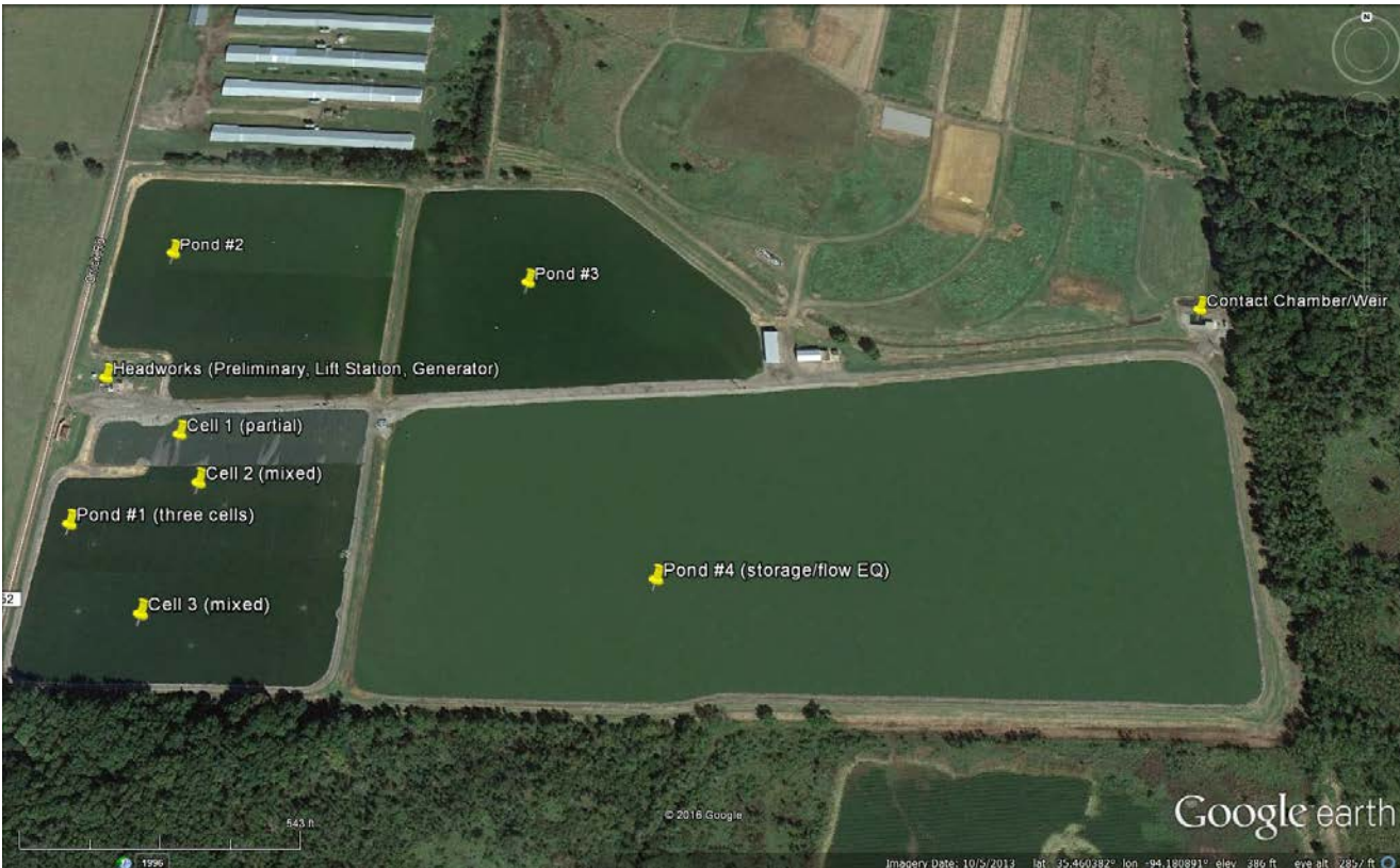
Figure 2. Google Earth image dated Oct 5, 2013 showing components of the City of Alma's WWTP.
