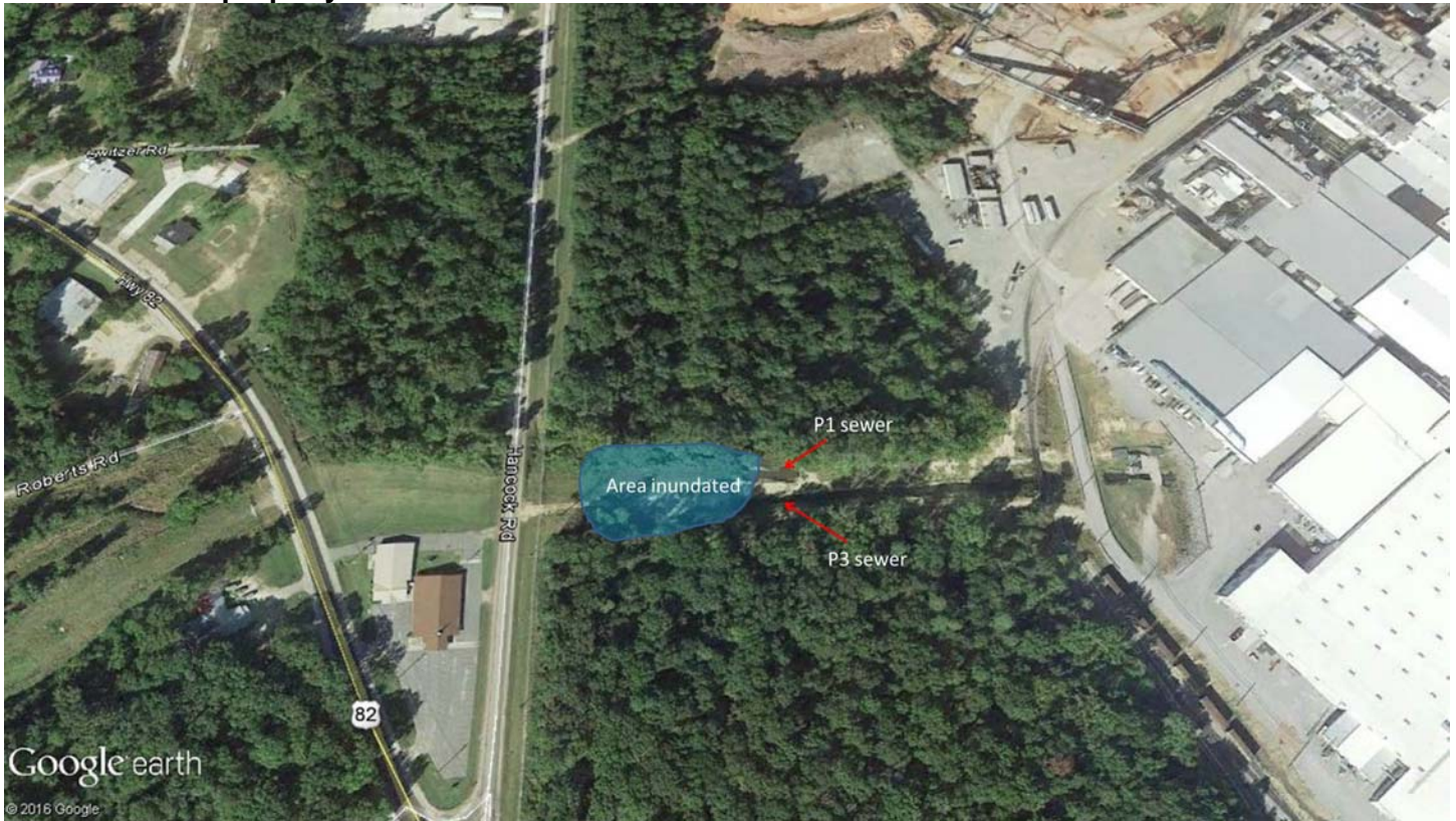
Figure 1. Overview of area directly west of Georgia-Pacific Crossett, LLC. The P1 and P3 sewer channels are labeled with arrows and the area shaded in blue was the area that was stated to have some inundation from flooding. It was unknown if commingled stormwater and untreated effluent made it off G-P property.
