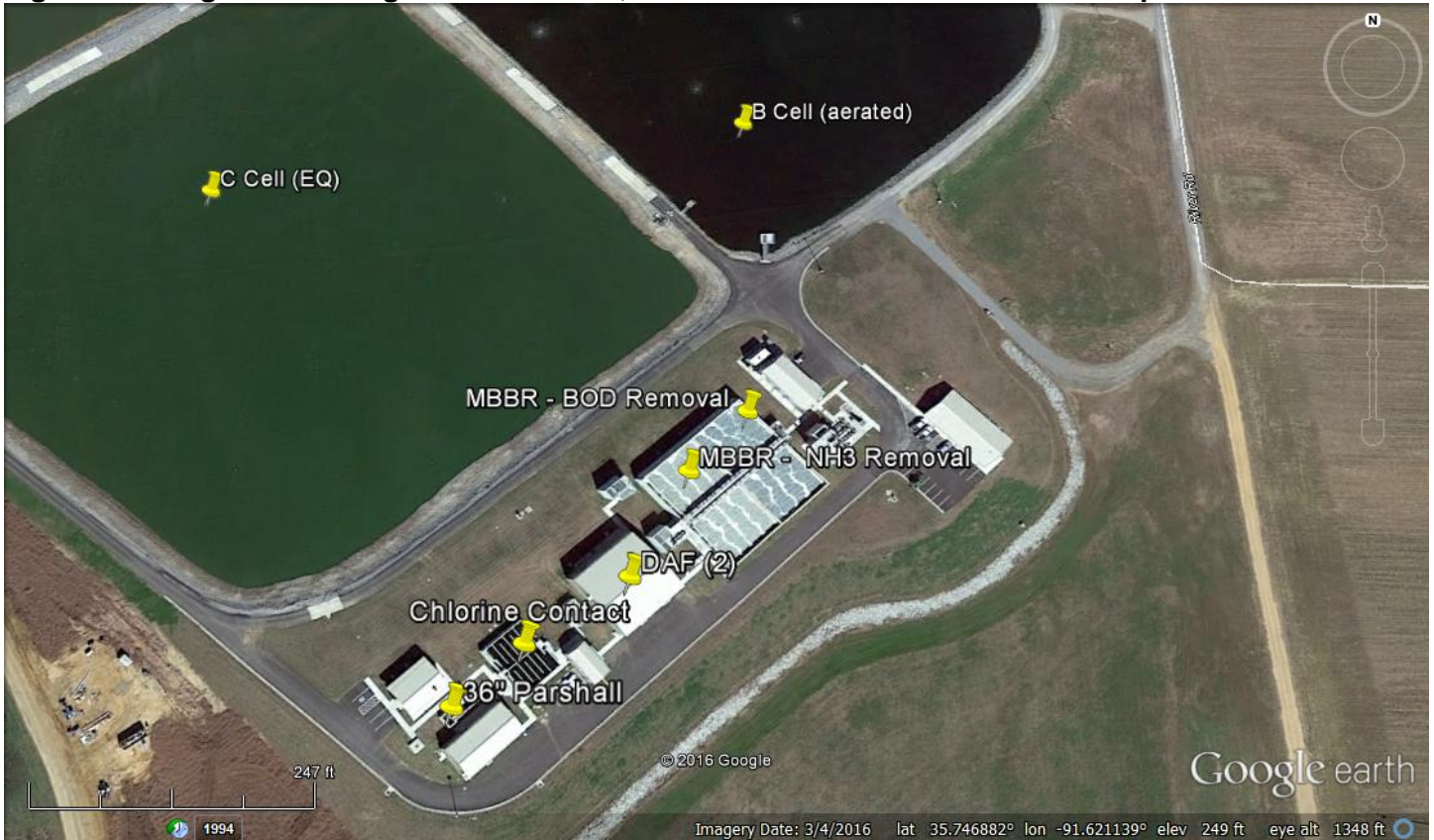
Figure 3. Google Earth image dated March 4, 2016 of MBBR and final effluent components.
