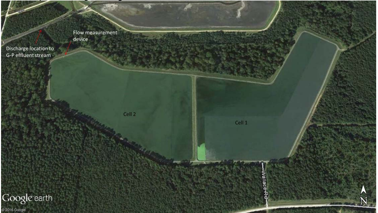
Figure 1. City of Crossett wastewater lagoons. Cell 1 has a baffle curtain installed throughout the entirety of the lagoon. Cell 2 has baffle curtains that separate the water into four (4) sections. Flow is measured prior to being discharged to G-P effluent stream.
