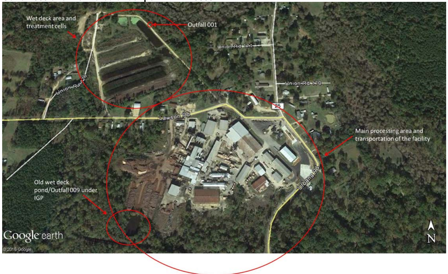
Figure 1. Overview of Anthony Forest Company – Urbana Sawmill. Indicated are the processing areas of the facility, the wet deck area, and the treatment cells. Also indicated is the location of Outfall 001. There is a pond on the south-side of the facility that is indicated that previously operated as a wet deck pond, but there is currently no process water being discharged from this pond. The pond is now Outfall 009 and monitored under permit ARR000977.
