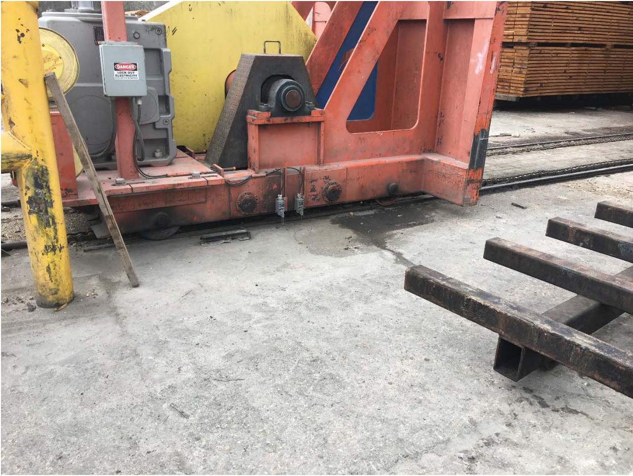
Photograph showing area in the vicinity of the kilns where excess grease has been observed.
