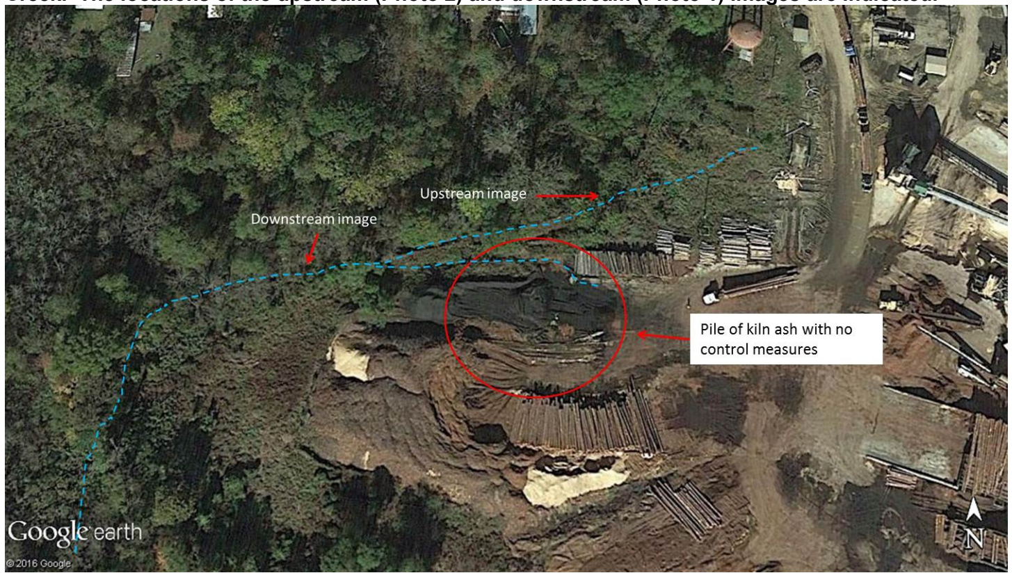
Figure 2. Drainage ditch that is had a lack of control measures and drains to Outfall 008. Control measures such as velocity dissipation devices and vegetation would adequately control wood chips and other materials from entering Woodard Creek.
