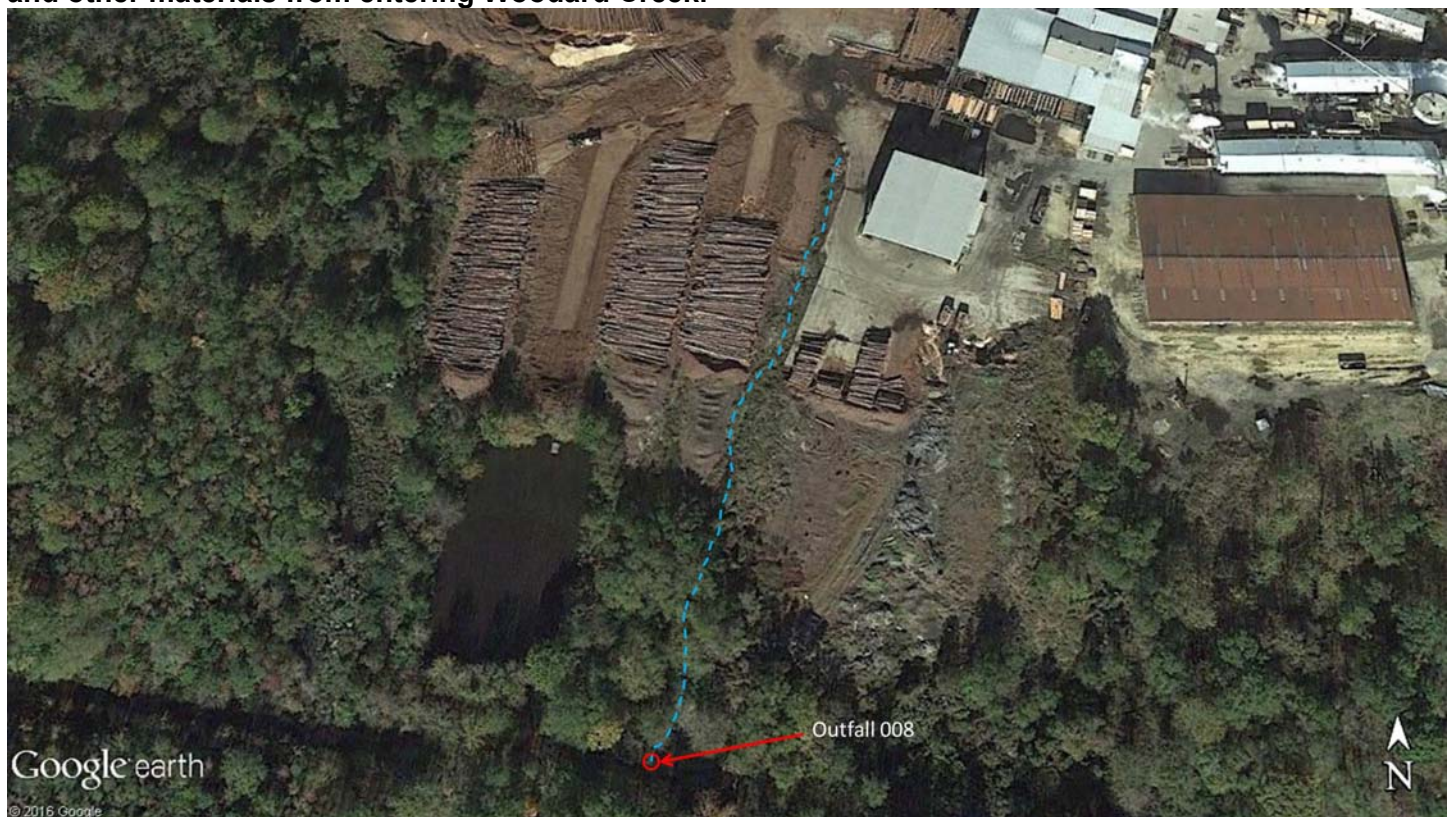
Figure 2. Drainage ditch that is had a lack of control measures and drains to Outfall 008. Control measures such as velocity dissipation devices and vegetation would adequately control wood chips and other materials from entering Woodard Creek.
