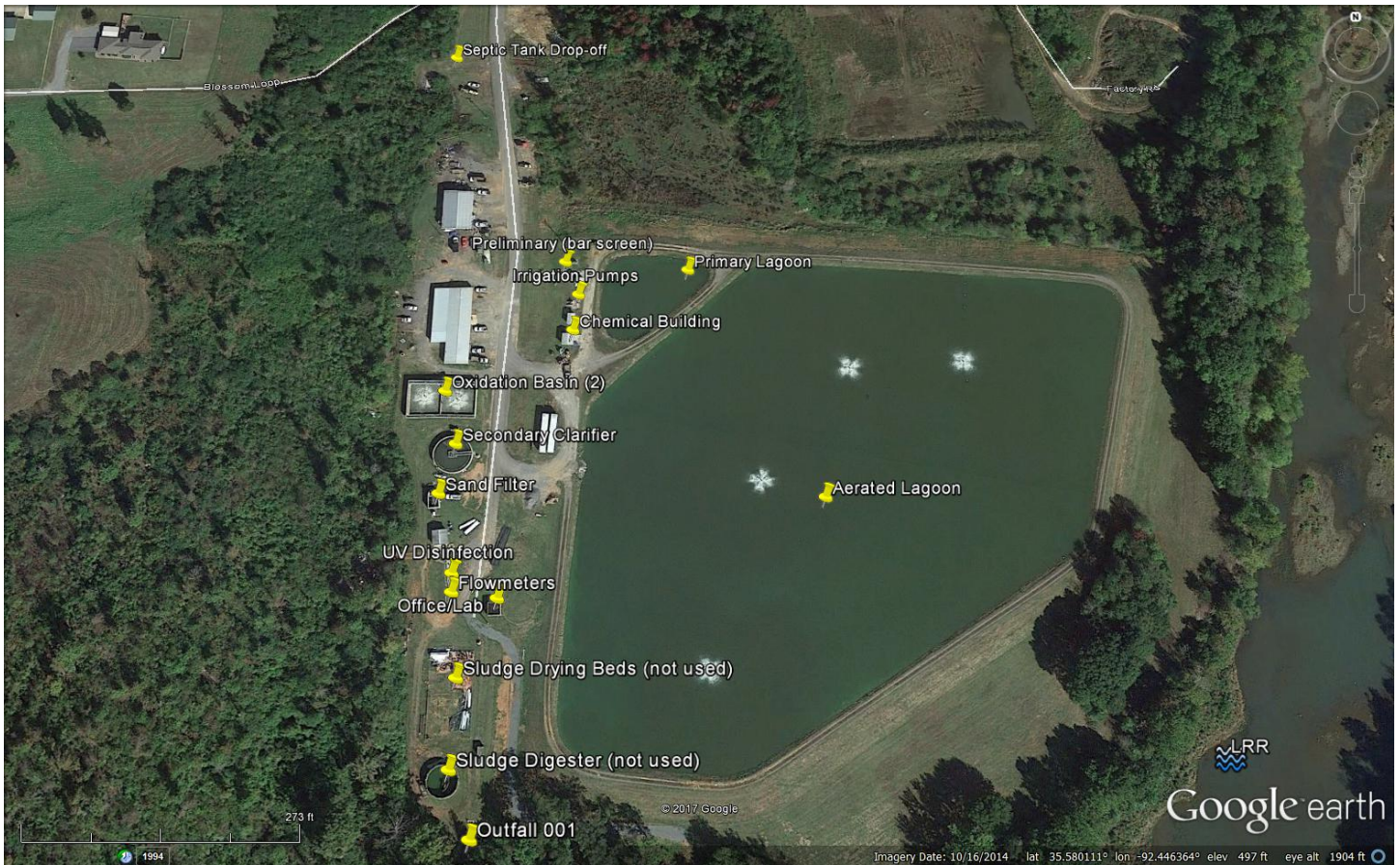
Figure 1. Google Earth image dated Oct 16, 2014 depicting City of Clinton (East Plant) with major components labeled.
