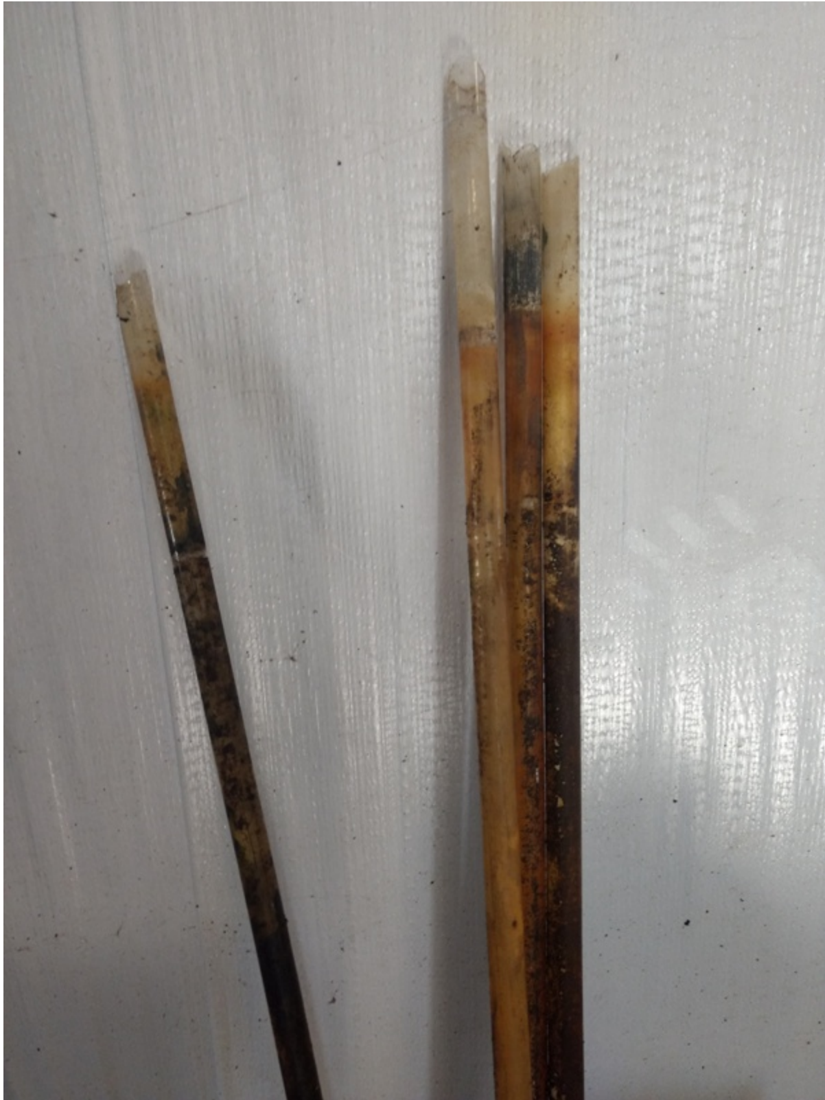
OLD QUARTZ SLEEVES EUREKA SPRINGS WWTP
