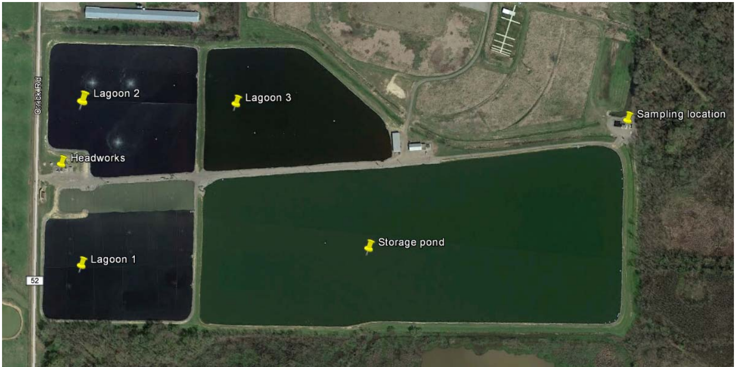
Figure 1. Google Earth image dated March 20, 2016 showing treatment components of the Alma WWTP.
