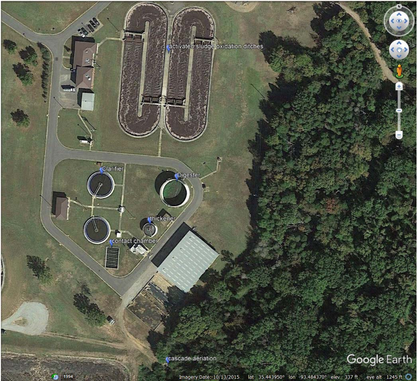
Figure 2. Google Earth image dated Oct 13, 2015 showing activated sludge (main) treatment plant and components.
