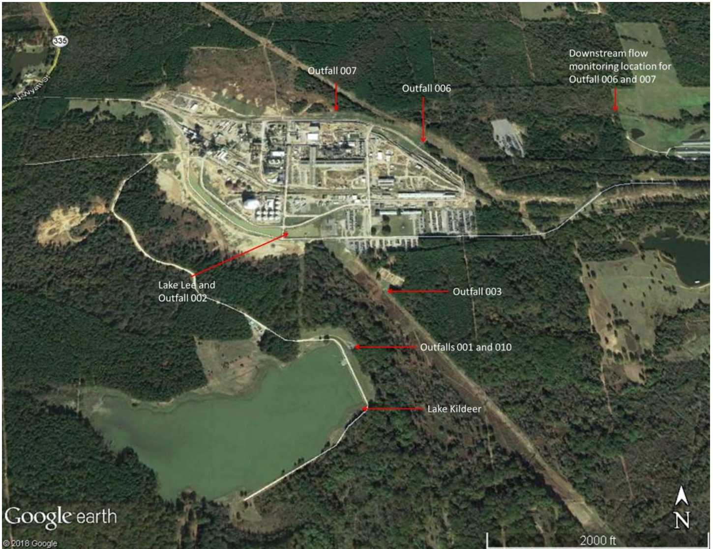
Figure 1. Overview of El Dorado Chemical Company with location of treatment lakes and outfalls identified.
