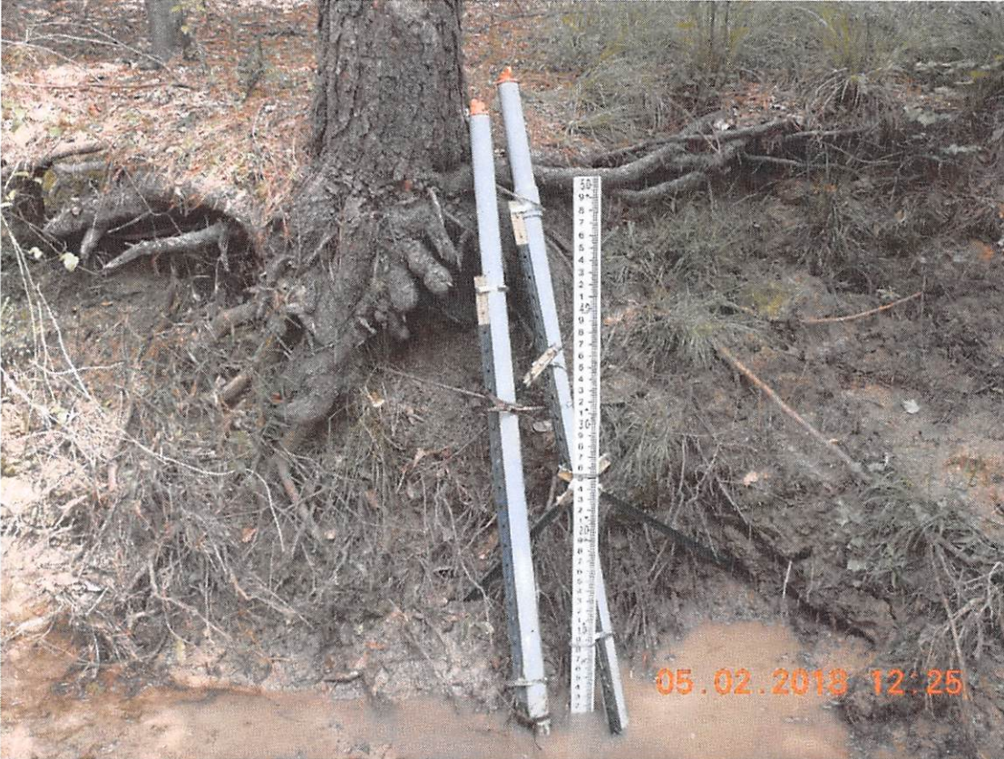
Photo #3 and #4: Back-up Level Logger and Staff Gauge at time of installation - May 02, 2018
