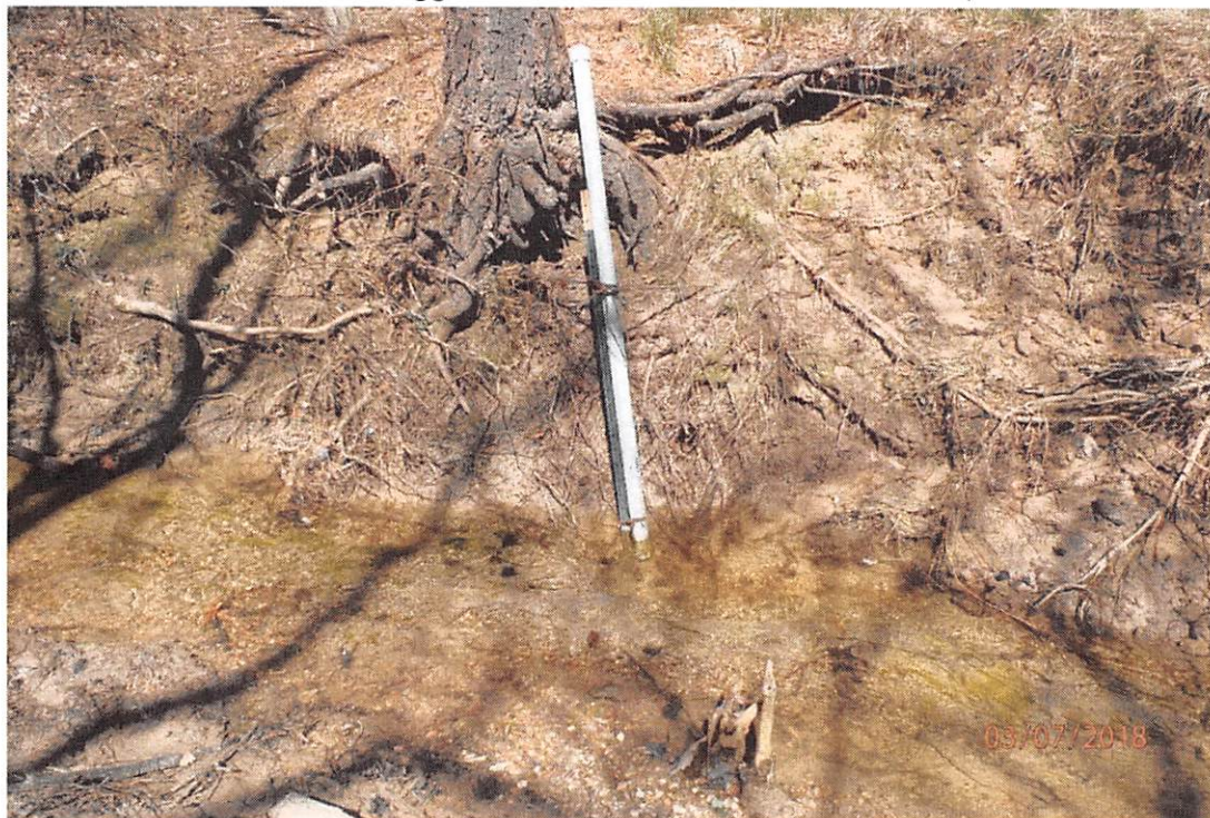
Photos #1 and #2: Level Logger at time of installation - March 07, 2018
