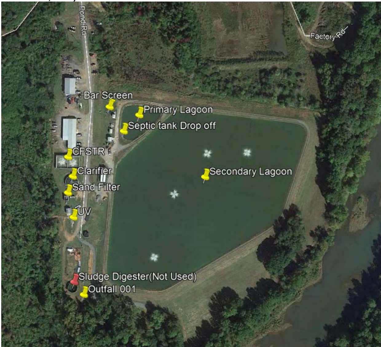
Figure 1. General overview of the site with major components labeled (Google Earth: imagery date October 16, 2014).
