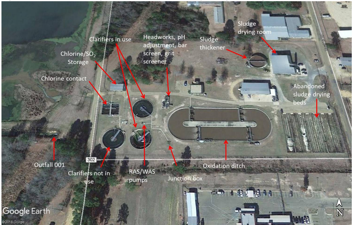
Figure 2. Overview of working components in WWTP at City of Magnolia – Big Creek WWTP.
