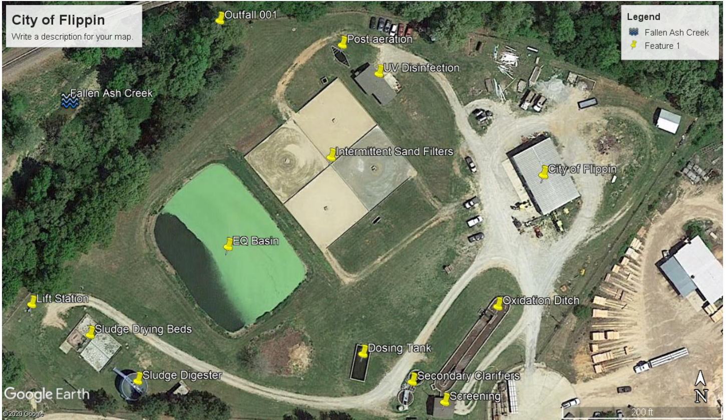
Figure 1. Google Earth image dated May 4, 2014 depicting the City of Flippin POTW with major components labeled.
