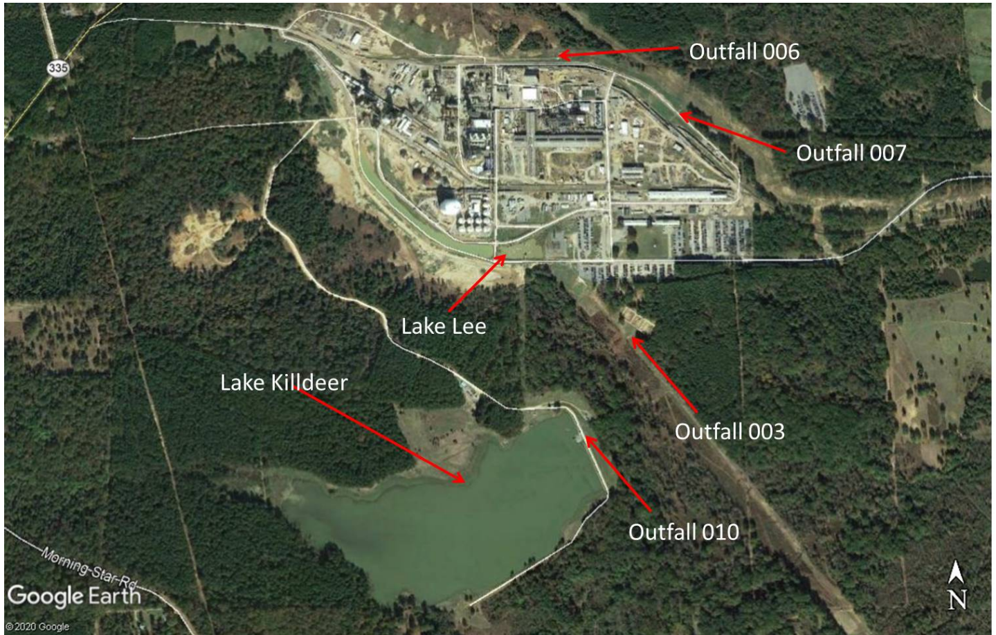
Figure 1. Overview of El Dorado Chemical and the location of treatment units and outfalls.
