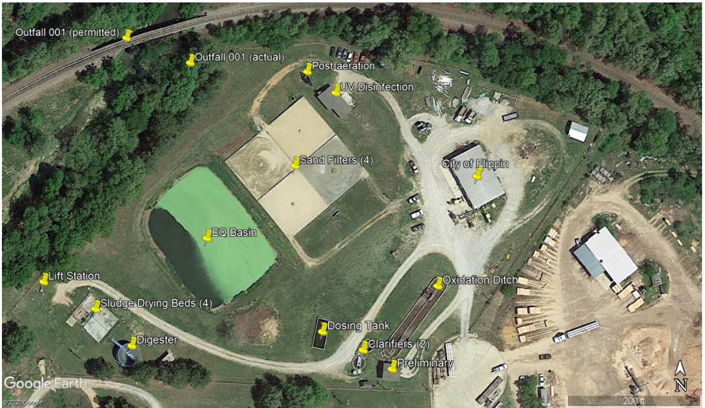
Figure 1. Google Earth image dated May 4, 2014 depicting City of Flippin POTW with major components identified.
