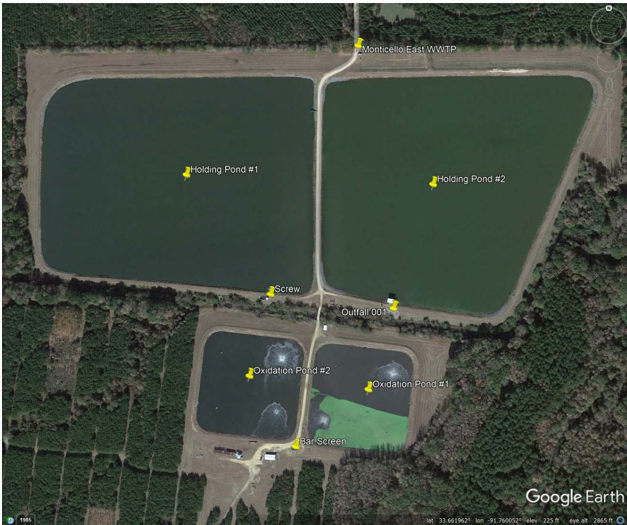
Figure 1. Google Earth aerial imagery dated Nov 14, 2019 showing the components of the facility.
