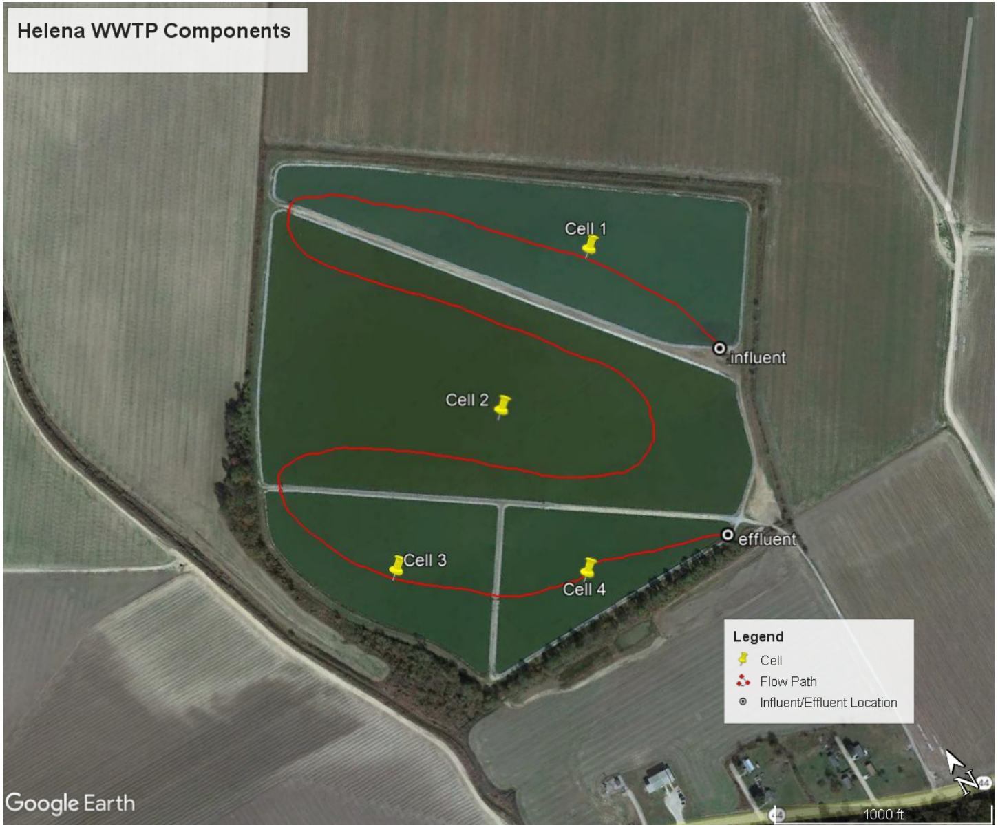
Figure 2. Google Earth image depicting components and simplified flow path of the Helena WWTP; satellite base imagery dated 11/11/2020.
