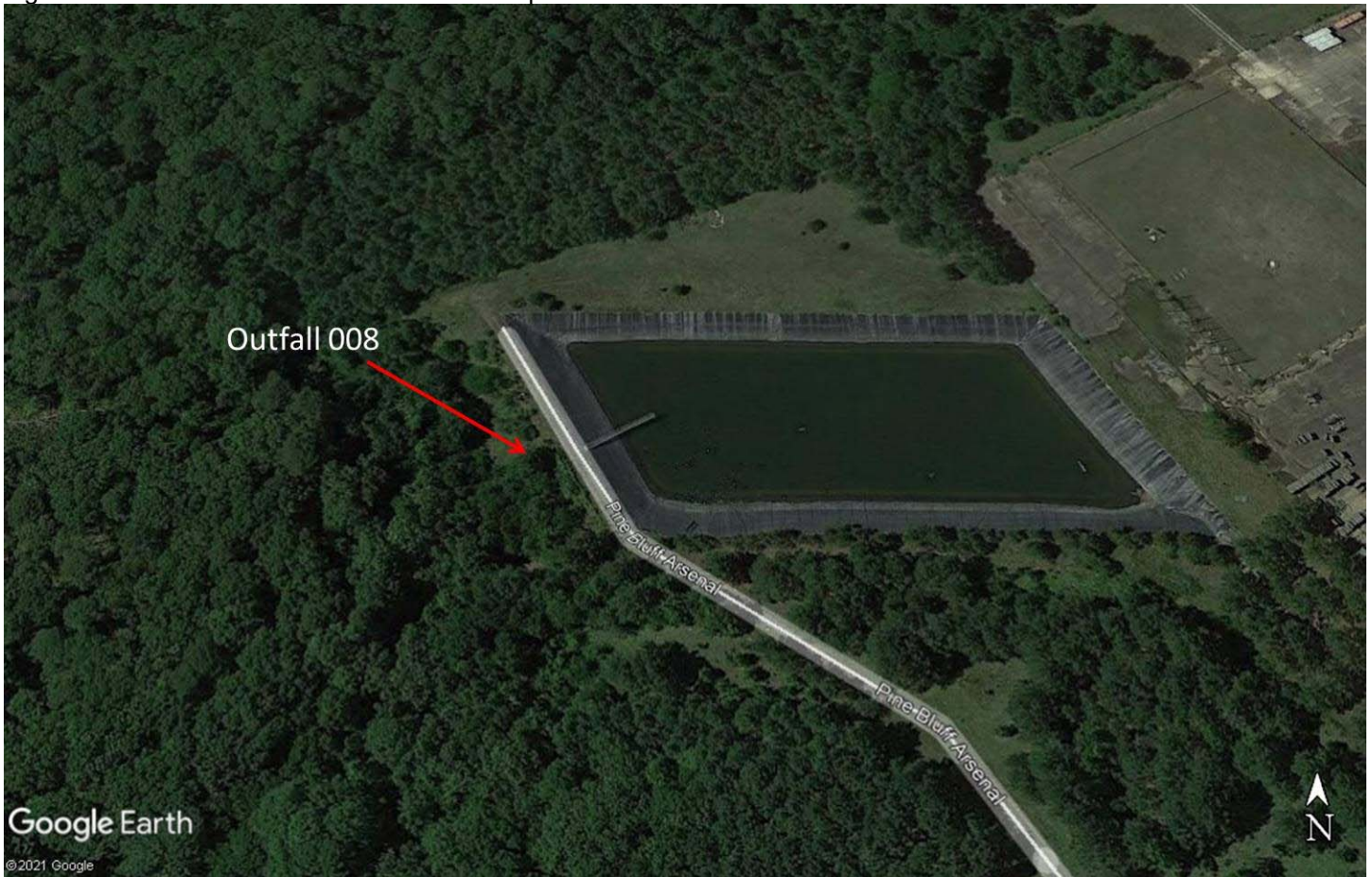
Figure 3. Location of Outfall 008 and the lined pond associated as treatment.
