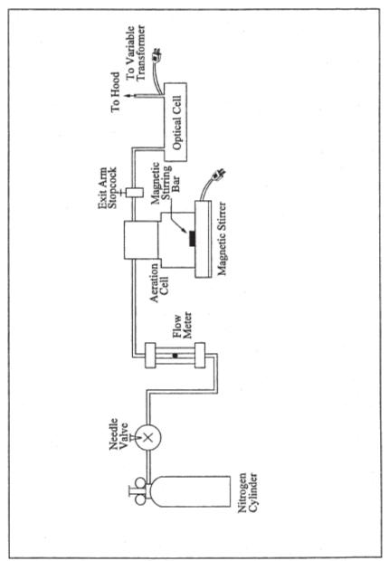
Figure 101-5. Schematic of Aeration System.
