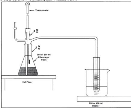
Figure 108C-1. Distillation Apparatus.
