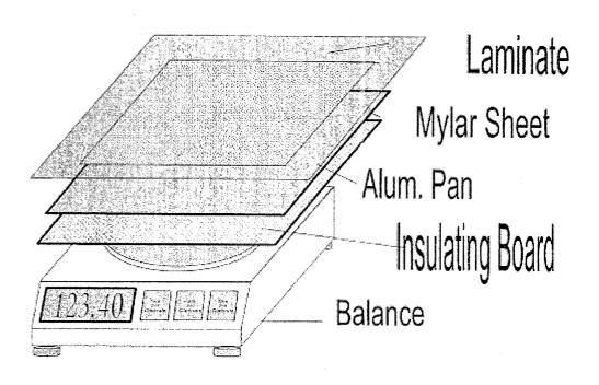
Figure 17.2. Scale, Place, Insulating Board, Mylar, Laminate Order
