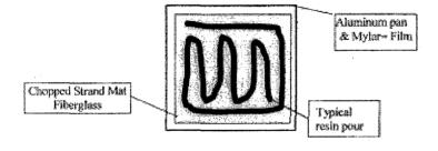
Figure 11.6 Resin Distribution Diagram
