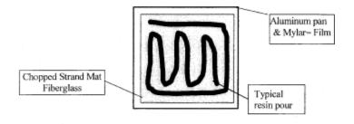
Figure 11.6 Resin Distribution Diagram
