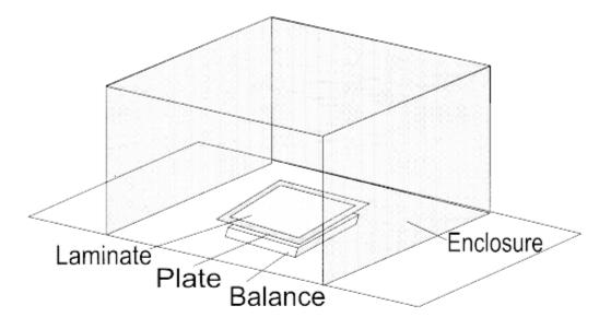
Figure 17.1. Typical Balance Enclosure
