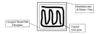
Figure 11.6 Resin Distribution Diagram
