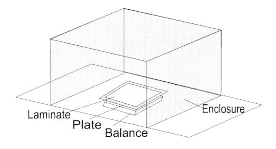
Figure 17.1. Typical Balance Enclosure
