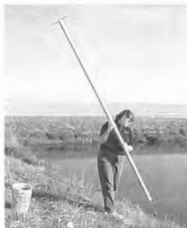
Figure 2. Sampling earthen basin with sampling probe.
