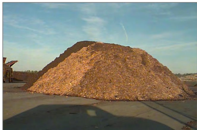
Boiler fuel is composed of ground hard and soft wood.
