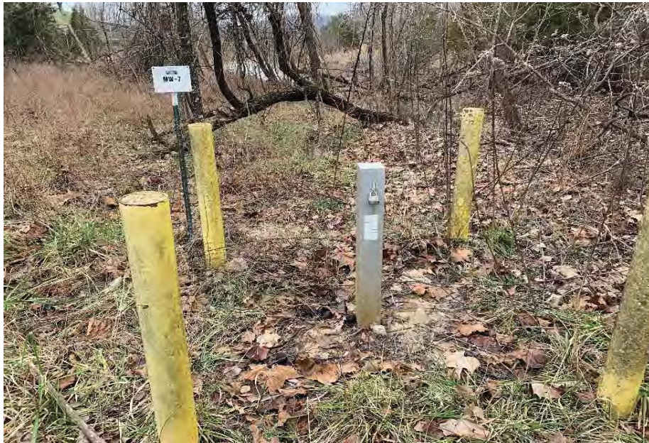
Photograph 15: Groundwater monitoring well MW-689 - locked.
