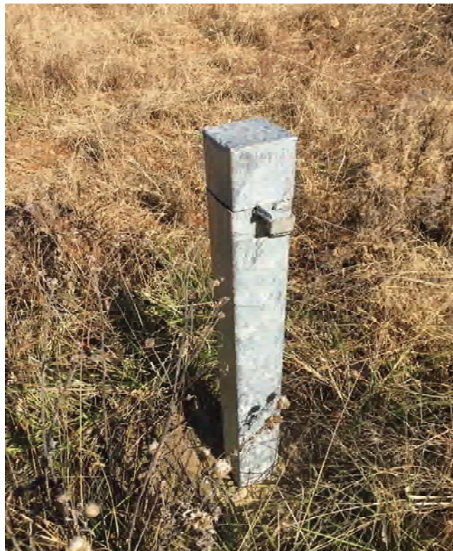
Photograph 21: Gas probe GP-18R - locked.
