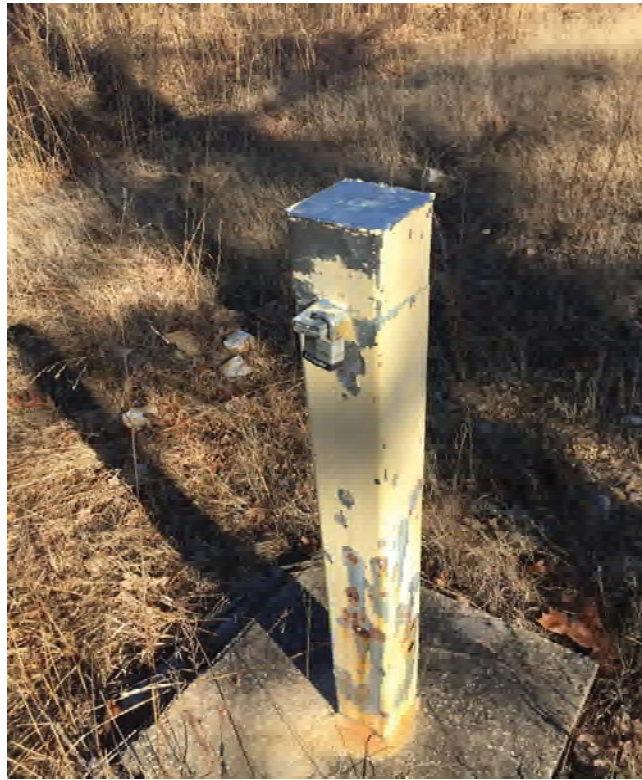
Photograph 3: Groundwater monitoring well CAO-3 - locked.
