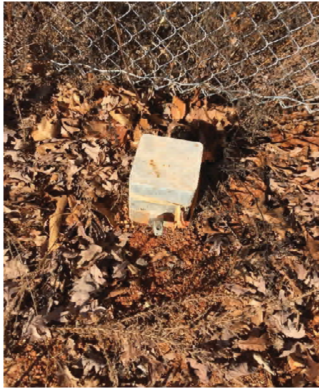
Photograph 17: Gas probe GP-16 - locked.
