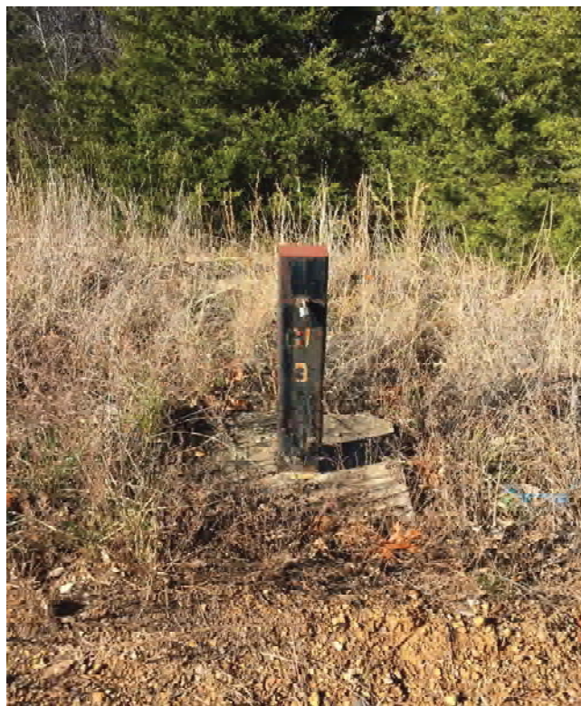
Photograph 3: Gas probe GP-3 - locked.
