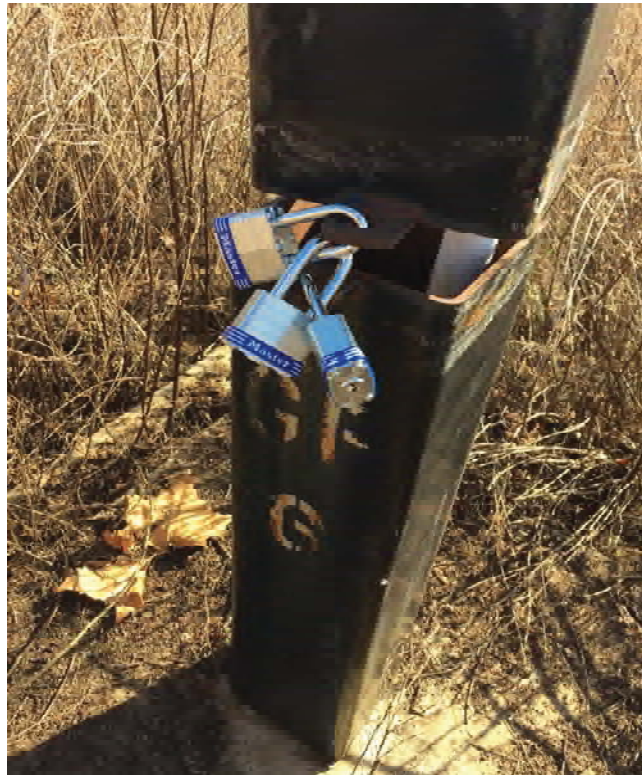
Photograph 6: Gas probe GP-6 - new daisy-chained locks added. Outer casing will not close properly due to extended inner well pipe.
