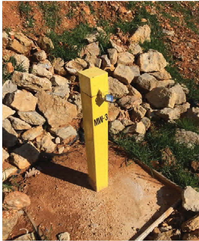
Photograph 7: Extended groundwater monitoring well MW-3 - new lock has been added.
