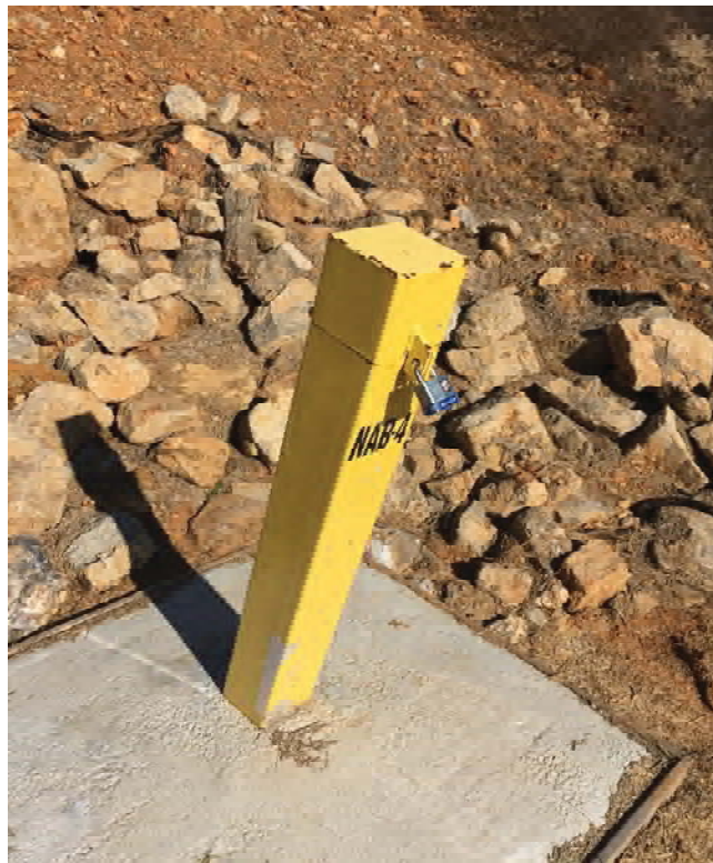
Photograph 18: Extended groundwater monitoring well NAB-4 - new lock has been added.
