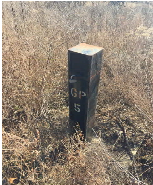
Photograph 5: Gas probe GP-5 - locked.
