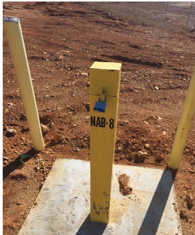
Photograph 20: Extended groundwater monitoring well NAB-8 - new lock has been added.
