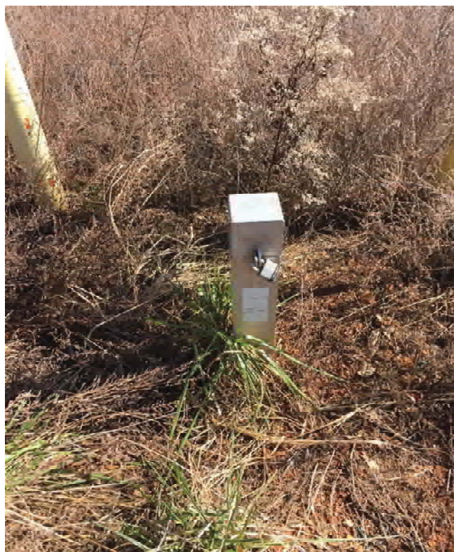
Photograph 6: Groundwater monitoring well MW-2 - locked.
