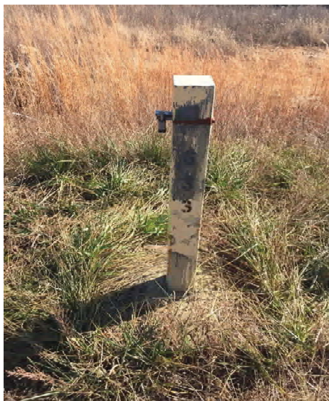
Photograph 13: Groundwater monitoring well MW-577 - locked.
