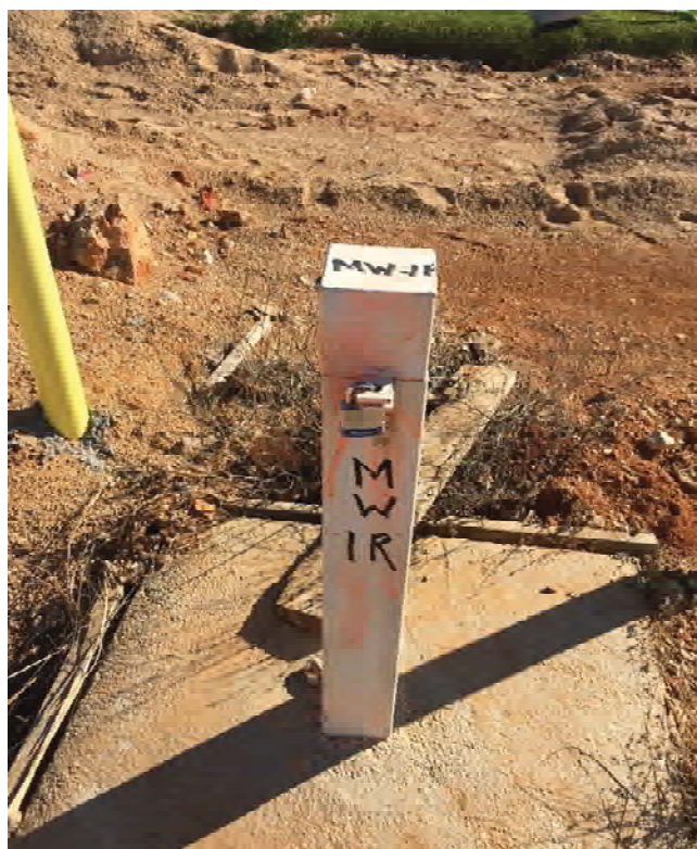
Photograph 5: Groundwater monitoring well MW-1R - locked.
