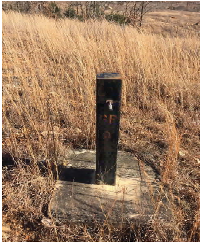
Photograph 9: Gas probe GP-9 - locked.
