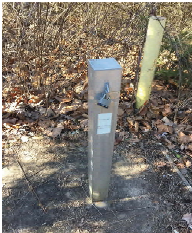
Photograph 12: Groundwater monitoring well MW-509 - locked.
