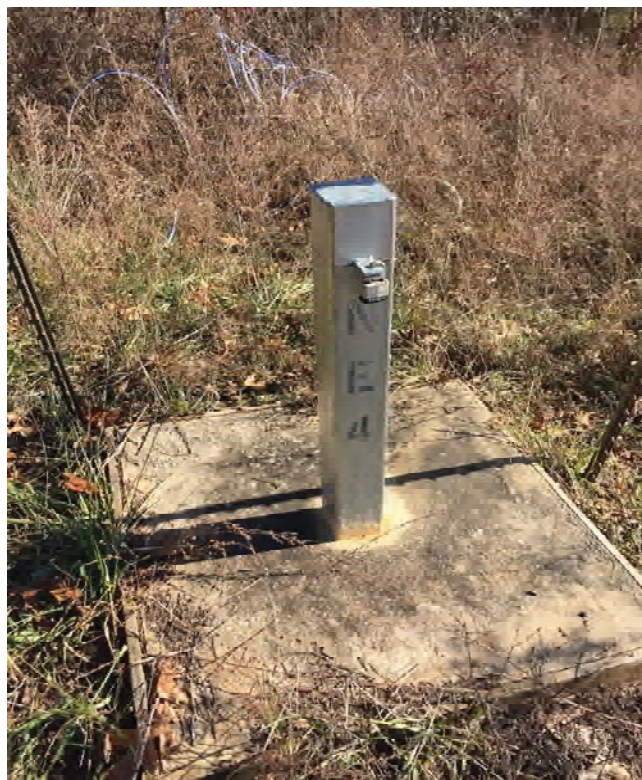
Photograph 23: Groundwater monitoring well NE-4 - locked.
