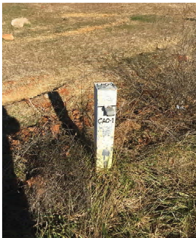
Photograph 1: Groundwater monitoring well CAO-1 - locked.
