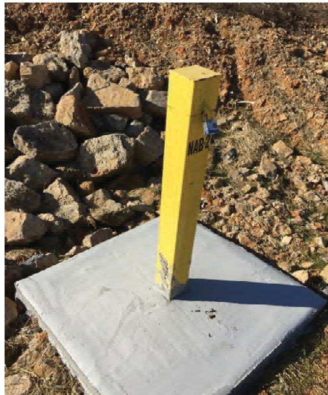
Photograph 16: Extended groundwater monitoring well NAB-2 - new lock has been added.
