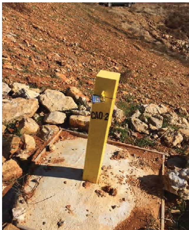
Photograph 2: Extended groundwater monitoring well CAO-2 - new lock has been added.
