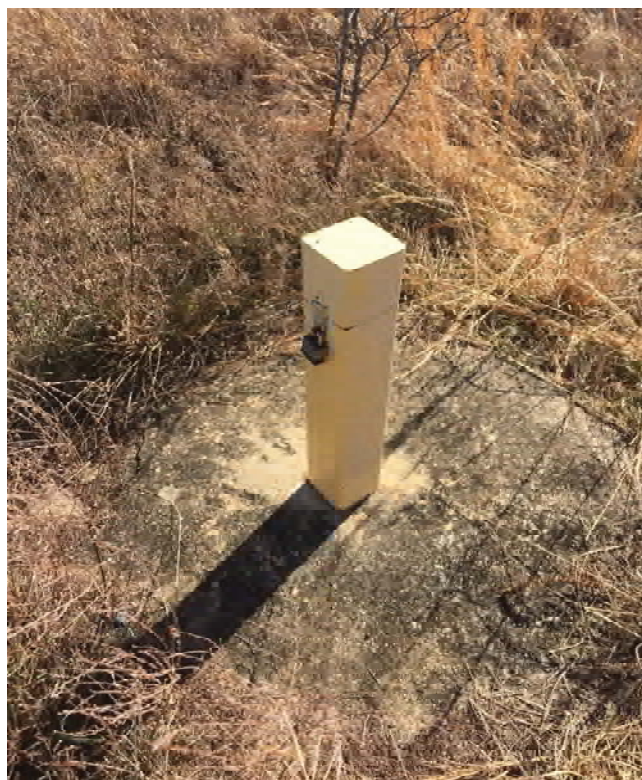
Photograph 14: Groundwater monitoring well MW-633 - locked.
