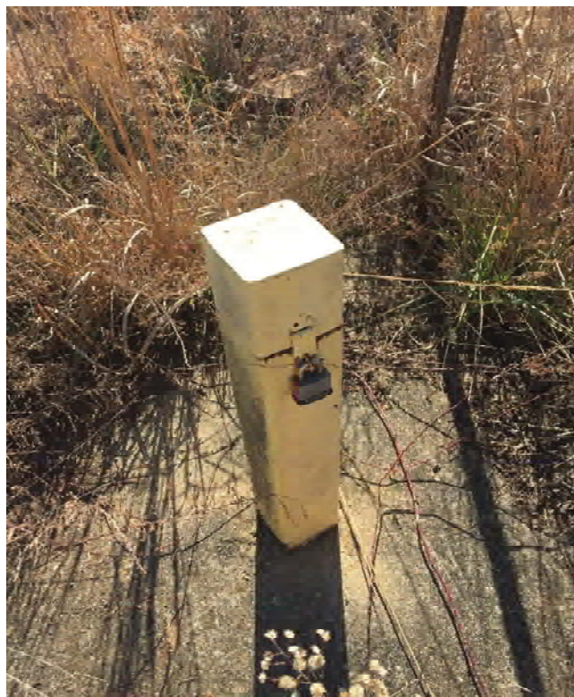
Photograph 11: Groundwater monitoring well MW-7 - locked.
