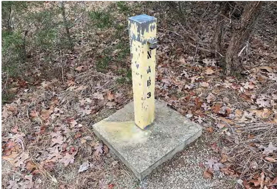
Photograph 17: Groundwater monitoring well NAB-3 - locked.
