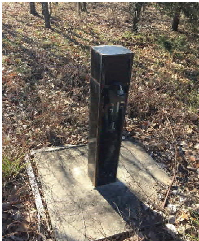
Photograph 4: Gas probe GP-4 - locked.
