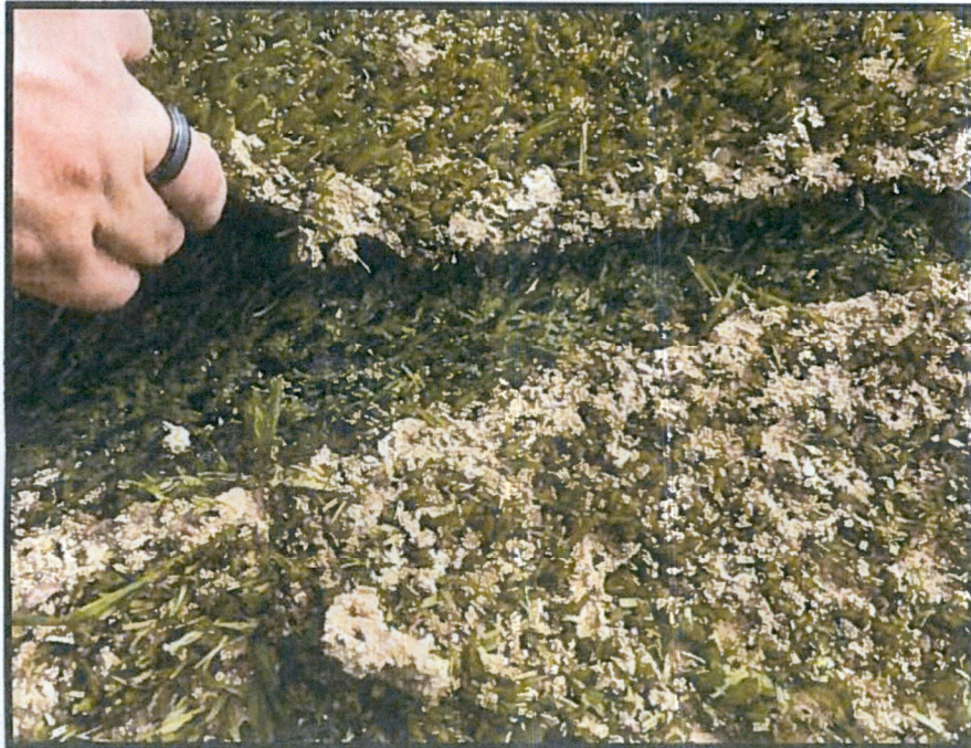
Photograph 11: Additional view of tear in ClosuresTurf®.
