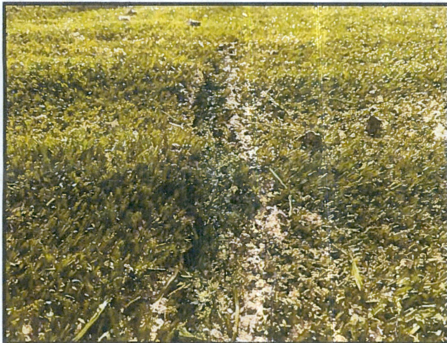
Photograph 12: Additional view of tear in ClosuresTurf®.
